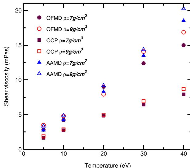
FIG. 4. The shear viscosity for  $C_2H_3$  mixture using the OFMD, OCP,<sup>31</sup> and AAMD methods as a function of temperature at the densities of  $7 \text{ g/cm}^3$  and  $9 \text{ g/cm}^3$ .
