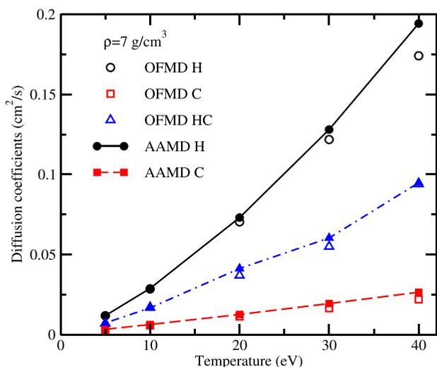
FIG. 2. The self- and mutual diffusion coefficients for  $C_2H_3$  mixture using the OFMD and AAMD methods as a function of temperature at the density of  $7 \text{ g/cm}^3$ . The self-diffusion coefficients for C are labeled by squares, and that for H labeled by circles, and triangles up represent the mutual diffusion coefficients.
