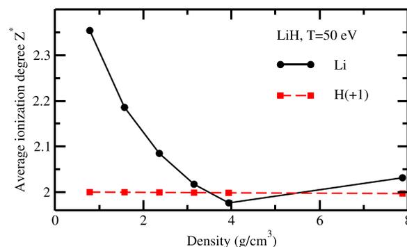
FIG. 7. The average ionization degree of Li and H in LiH mixture using modified AA method as a function of density at the temperature of 50 eV. Solid line with cycles is the results of Li and dashed line with squares is that of H. In order to show the results of H and Li in the same figure, the results of H have been plus 1.
