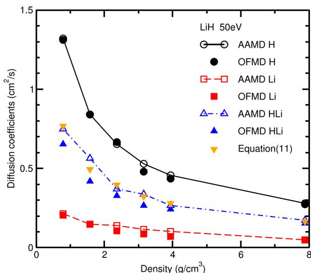
FIG. 5. The self- and mutual diffusion coefficients for LiH mixture using the OFMD and AAMD methods as a function of density at the temperature of 50 eV. Triangles down represent the data calculated from the self-diffusion coefficients  $C$  and  $H$  with Eq. (11).
