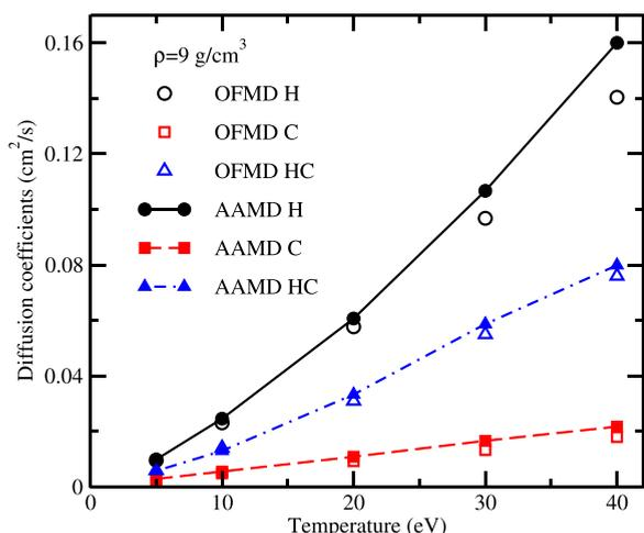
FIG. 3. The self- and mutual diffusion coefficients for  $C_2H_3$  mixture using the OFMD and AAMD methods as a function of temperature at the density of  $9 \text{ g/cm}^3$ . The self-diffusion coefficients for C are labeled by squares, and that for H labeled by circles, and triangles up represent the mutual diffusion coefficients.
