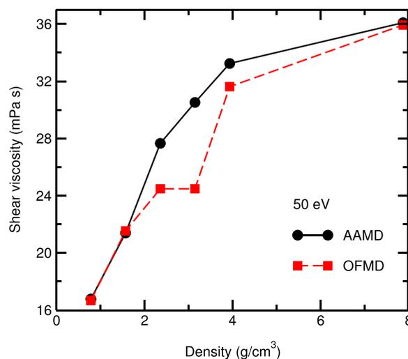
FIG. 6. The shear viscosity for LiH mixture using the OFMD<sup>32</sup> and AAMD methods as a function of density at the temperature of 50 eV.
