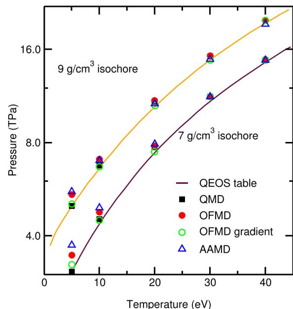
FIG. 1. Pressure versus temperature for  $C_2H_3$  mixture along the two isochores,  $7\text{ g/cm}^3$  and  $9\text{ g/cm}^3$  calculated by different methods: QMD (square), OFMD (circle), AAMD (triangle), and QEOS (line) table.
