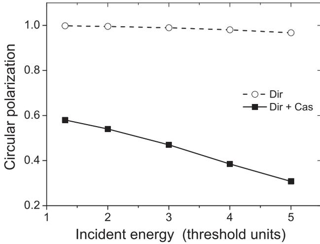
**Figure 4.** Circular polarization of the  $1s2s_{1/2} (J = 1) \rightarrow 1s^2 (J = 0)$  line of He-like  $\text{Fe}^{24+}$  ions as a function of the incident energy. Here, Dir represents the direct results without cascade contributions, and Dir + Cas the results with the latter included.
