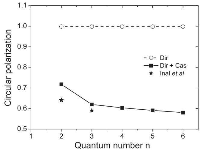
**Figure 3.** Circular polarization of the  $1s2s_{1/2}$  ( $J = 1$ )  $\rightarrow 1s^2$  ( $J = 0$ ) line of He-like  $\text{Fe}^{24+}$  ions as a function of the quantum number  $n$ . Here, Dir represents the direct results without cascade contributions, and Dir + Cas the results with the latter included. The stars represent the semirelativistic results obtained by Inal *et al* [15].
