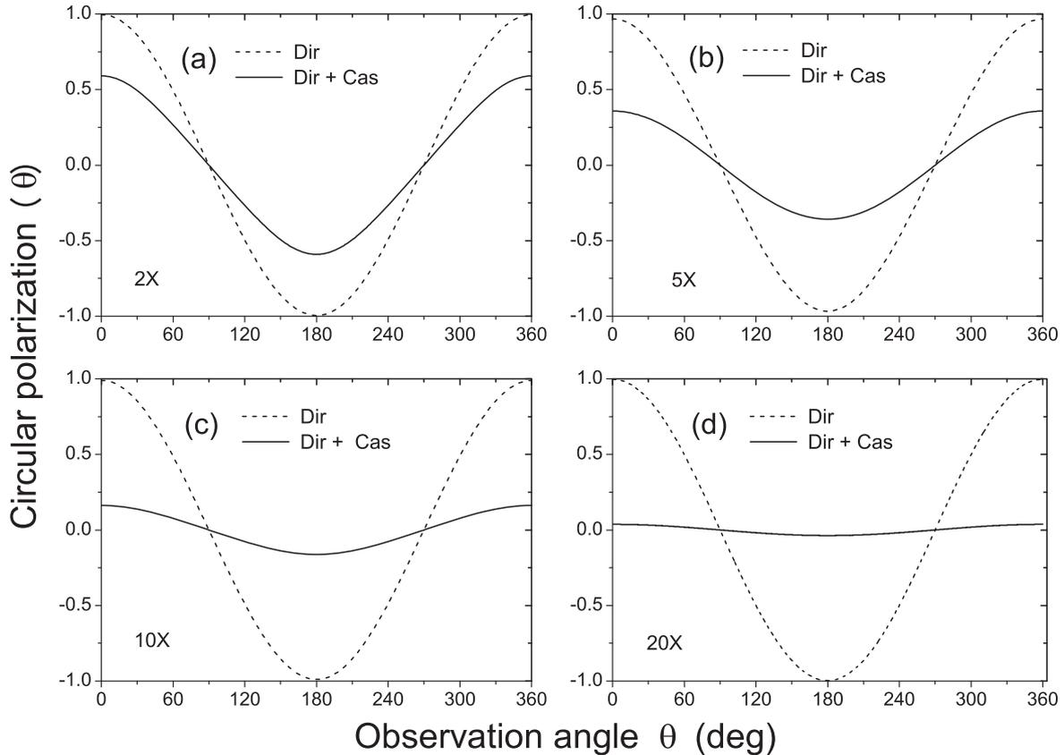
**Figure 5.** Angular distribution of the circular polarization for the  $1s2s_{1/2} (J = 1) \rightarrow 1s^2 (J = 0)$  line of He-like  $\text{Fe}^{24+}$  ions as a function of the observation angle for incident energies of: (a) 2, (b) 5, (c) 10, and (d) 20 times the threshold energy X. Here, Dir represents the direct results without cascade contributions, and Dir + Cas the results with the latter included.
