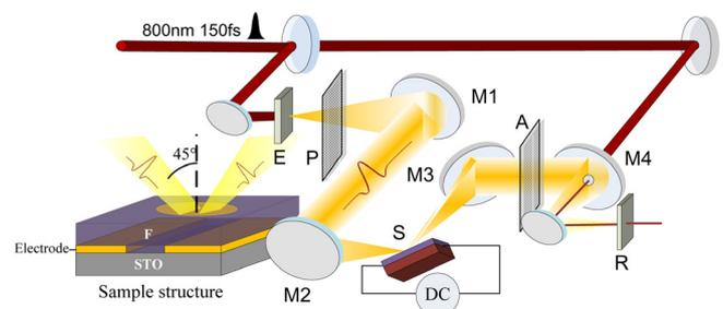
FIG. 1. The schematic diagram of THz-TDS for measuring the electro-optic effects in sample films. E: THz emitter, R: THz receiver, S: sample, M1 ~ M4: parabolic mirrors, P: THz polarizer, A: THz analyzer, DC: direct current source. The inset is the structure diagram of the sample. F: ferroelectric film.
