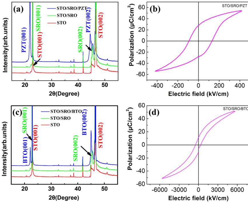
FIG. 2. The properties characterized by XRD and RT Precision workstation. The XRD patterns of PZT (a) and BTO (c) films; The P-E curves of PZT (b) and BTO (d) thin films.
