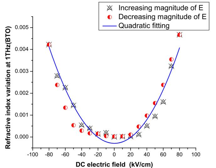
FIG. 4. Electro-optic response of the (001)-oriented BTO thin film in an external electric field of up to 80 kV/cm. Black triangle dots are experimental value of field increasing process. Red circle dots are experimental value of field decreasing process. Blue line is the polynomial fitting curve.
