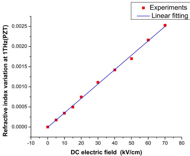
FIG. 3. Field induced birefringence of the (001)-oriented PZT thin film in an external electric field of up to 70 kV/cm. Red square dots are the experimental value. Blue line is the linear fitting curve.
