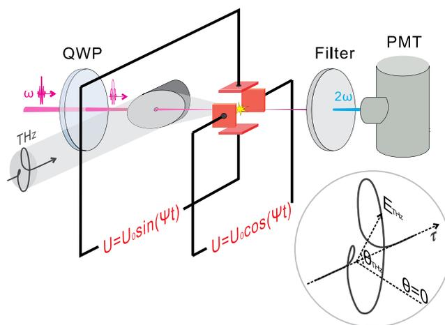
FIG. 1. The scheme of polarization-sensitive ABCD. QWP: broadbandwidth quarter wave plate; PMT: photomultiplier tube.
