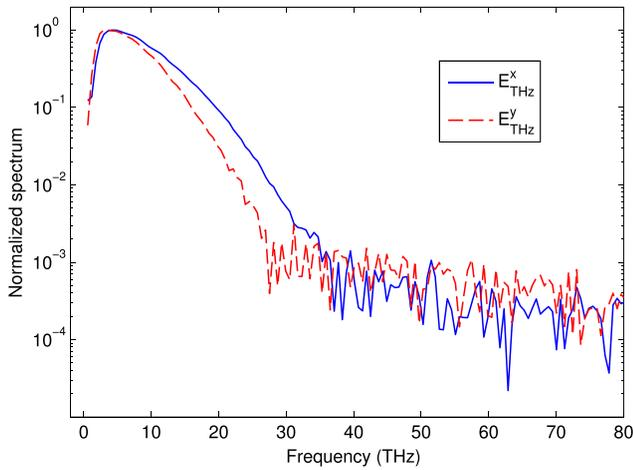
FIG. 4. The normalized spectra of the two orthogonal components of THz field.
