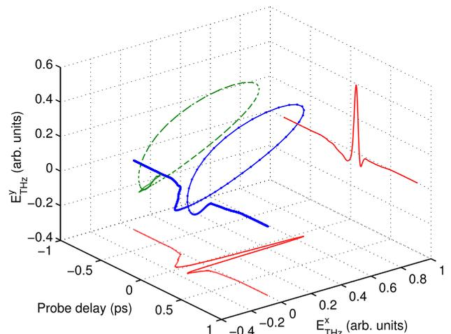
FIG. 3. The measuring result of an elliptical polarized THz wave. The orthogonal components and the polarization information are also shown as cast shadows in the figure.
