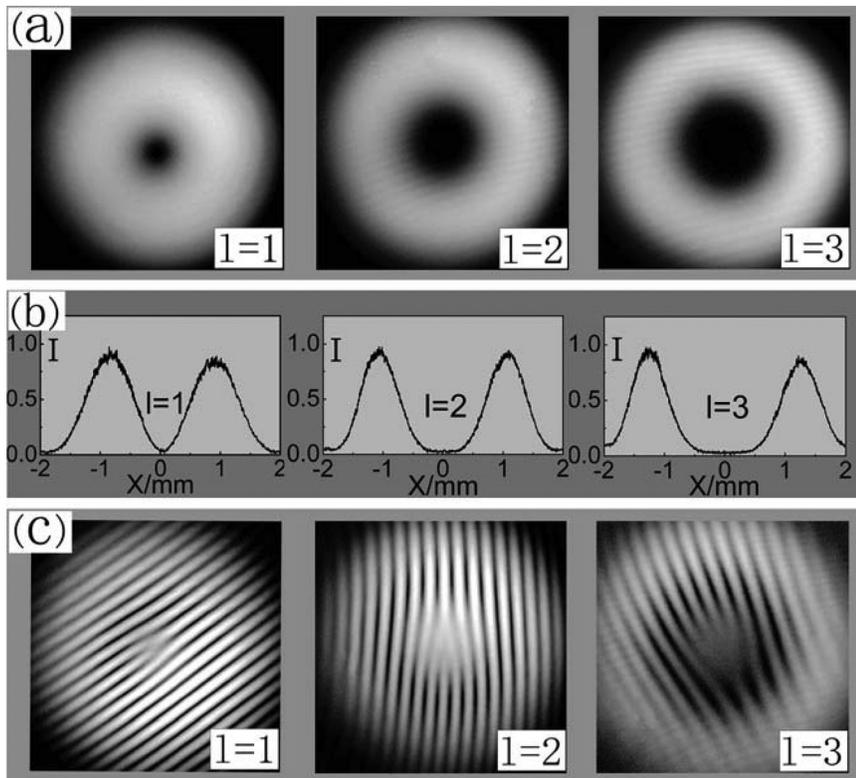
FIG. 4. (a) The  $LG_0^l$  mode obtained from the +1 order diffraction of the CGH gratings with different charges ( $l=1, 2, 3$ ); (b) the normalized transverse intensity distribution of  $LG_0^l$  beams corresponding to (a); (c) the interference patterns of the  $LG_0^l$  beams and the reference Gaussian beam.
