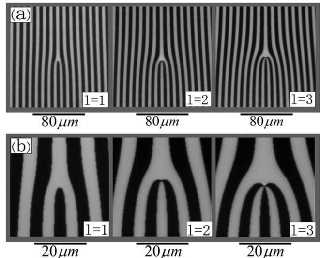
FIG. 3. The structures of CGH gratings with charges of  $l = 1, 2, 3$  observed under microscope. (a) and (b) display the central forks observed under different magnifications.
