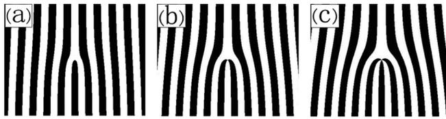
FIG. 1. Binary CGH grating patterns: (a)  $l = 1$ ; (b)  $l = 2$ ; and (c)  $l = 3$ . The fork reveals the phase singularity.
