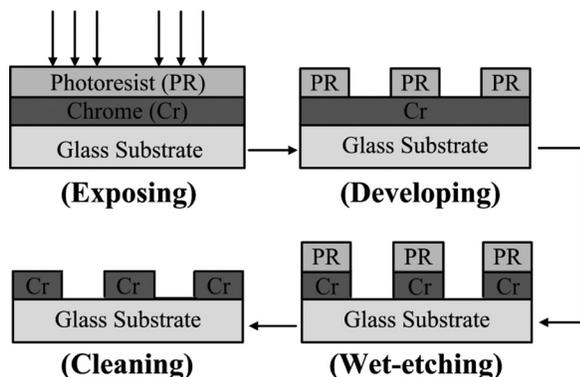
FIG. 2. The CGH grating fabrication by photolithography.
