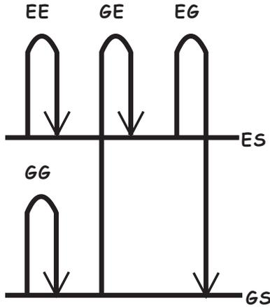
**Figure 4.** Illustration of HHG pathways. When molecules are coherently populated in two states indicated by GS and ES, there are four possible paths contributing to HHG labelled based on which states the electron is released and into which states it recombines.
