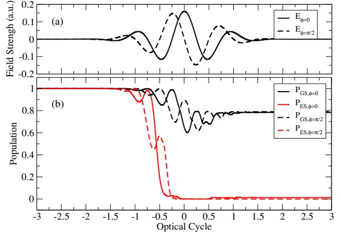
**Figure 1.** (a) Instantaneous electric fields for CEPs of 0 (solid lines) and  $\frac{\pi}{2}$  (dashed lines). (b) Population in the initial states for molecules prepared in the electronic ground state (black lines) and the first excited state (red lines) subjected to a laser pulse with CEPs of 0 (solid lines) or  $\frac{\pi}{2}$  (dashed lines), respectively.
