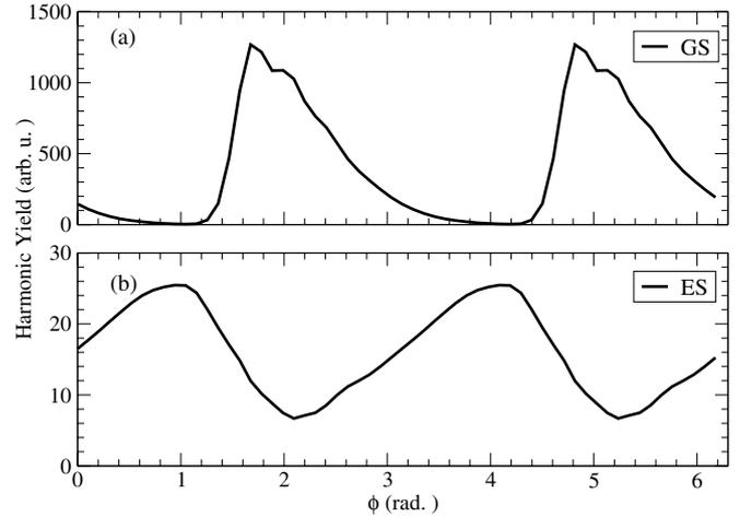
**Figure 3.** Integrated spectral yields over harmonic order of 110 and 150 versus CEPs of the laser pulse from molecules prepared in (a) the electronic ground state and (b) the first excited state.
