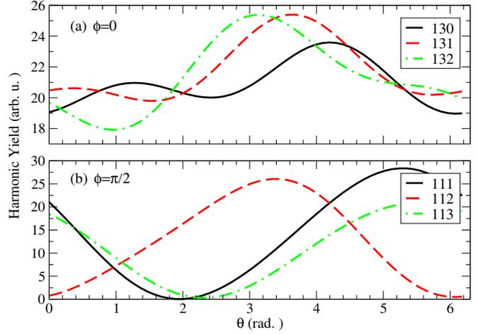
**Figure 5.** Variation of harmonic intensity with the initial phase  $\theta$  for laser CEP of (a)  $\phi = 0$  and (b)  $\phi = \frac{\pi}{2}$  for the given harmonic orders labelled. The molecules are prepared in a coherent superposition of the ground state and the first excited state with a population ratio of 1 : 1.
