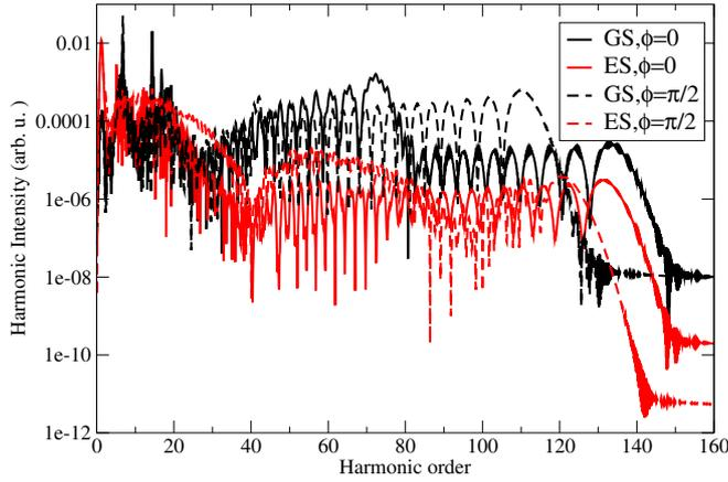
**Figure 2.** Harmonic spectra from molecules prepared in the electronic ground state and the first excited state subject to laser pulses of CEP 0 and  $\frac{\pi}{2}$ .
