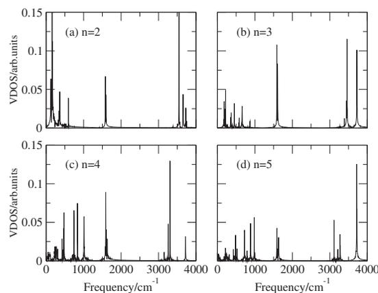
FIG. 3. The calculated vibrational density of states for the ground state  $(\text{H}_2\text{O})_n$  ( $n=2-5$ ) clusters.
