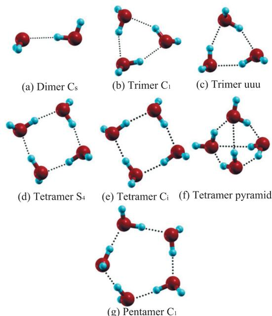
FIG. 1. Structures of  $(\text{H}_2\text{O})_n$  ( $n=2-5$ ). (a), (b), (d), and (g) are the ground-state structures of  $(\text{H}_2\text{O})_n$  ( $n=2-5$ ), respectively. (c) is one of trimer isomers. (e) and (f) are two tetramer isomers. The dotted lines denote the H-bonds.
