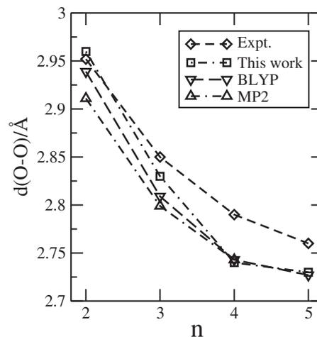
FIG. 2. Comparison of the computed OO distances in water clusters through various methods with the experimental value. The results of BLYP, MP2, and experiment are from Refs. 54, 42, and 22, respectively.
