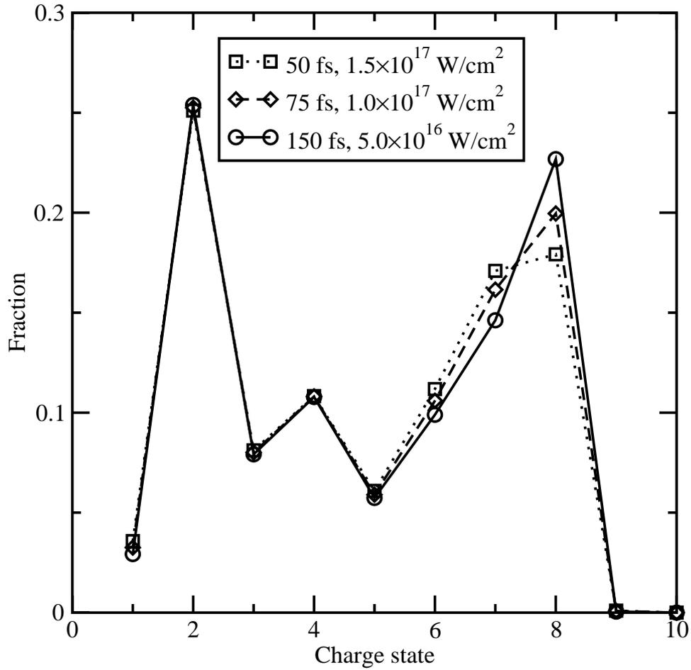
Figure 4: CSD of neon irradiated by x-ray pulses with the same value of  $I_0 \times \tau$ , i.e., 50 fs and  $1.5 \times 10^{17}$  W/cm<sup>2</sup> (dotted line with squares), 75 fs and  $1.0 \times 10^{17}$  W/cm<sup>2</sup> (dashed line with diamonds) and 150 fs and  $5.0 \times 10^{16}$  W/cm<sup>2</sup> (solid line with circles), respectively. The central photon energy of the x-ray pulse is  $h\nu_0=1110$  eV.
