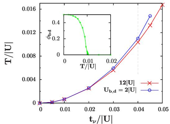
FIG. 3: Critical temperature of the PSF as a function of hopping amplitudes  $t_b = t_d$  on a 3D cubic lattice with total filling  $n = 1$ . Inset: melting of the PSF vs. temperature along the vertical dashed line with hopping amplitudes  $t_b = t_d = 0.04|U|$ .
