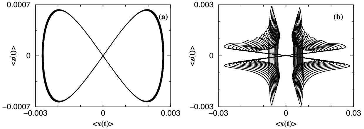
**Figure 2.** The electronic trajectory calculated from the TDDE for the ion with potential  $V(x, z) = -24/\sqrt{x^2 + z^2 + 0.001}$ . The frequency and the electric strength are set to  $\omega = 1.0$  au and (a)  $E = 100$  au and (b)  $E = 300$  au.
