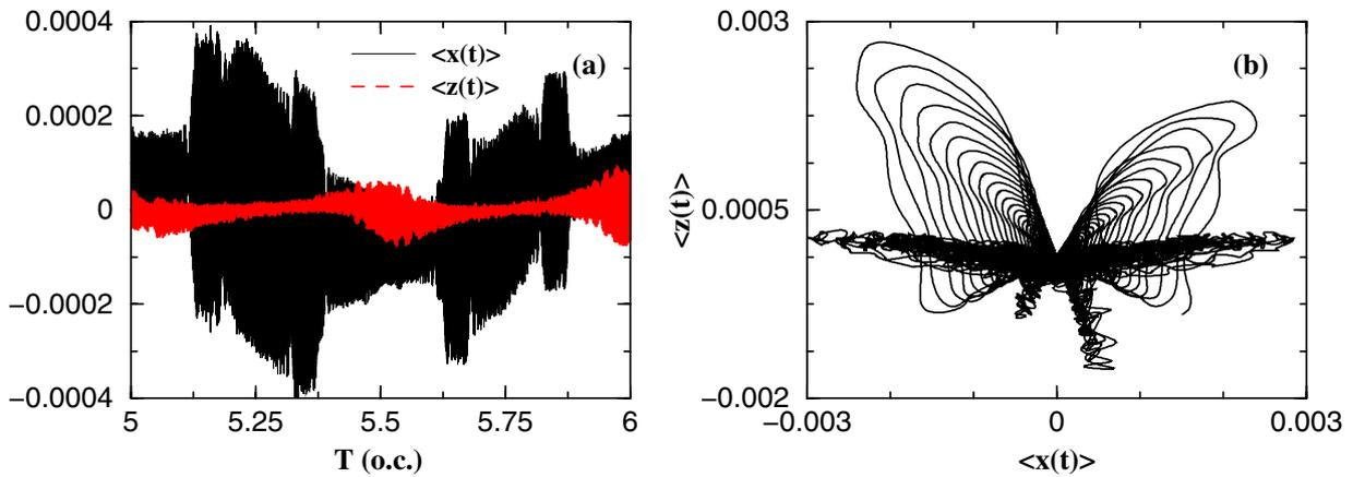
**Figure 3.** (a) The time-dependent displacement in the polarization (black solid line) and the propagation direction (red dashed line) for the ionic model  $V(x, z) = -79/\sqrt{x^2 + z^2 + 10^{-4}}$ . The frequency and the electric strength are set to  $\omega = 1.0$  au and  $E = 500$  au, respectively. (b) The electronic trajectory in the laser field of  $\omega = 10.0$  au and  $E = 3500$  au.
