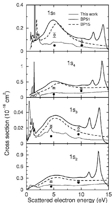
FIG. 3. The excitation cross sections from the ground level to the levels of  $4p^5 5s$  configuration as a function of scattered electron energy (solid lines, this work). The dotted lines represent 51-state BP *R*-matrix calculation obtained by Dasgupta *et al.* [18]; dashed lines, 15-state BPRM results [18]. The experimental data are from Trajmar *et al.* [3] (solid circles) and Guo *et al.* [8] (open circles).
