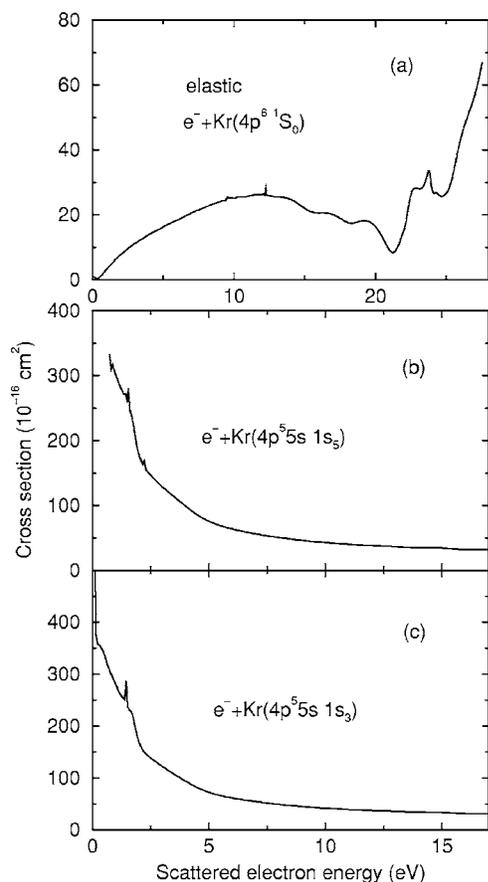
FIG. 2. The elastic scattering cross sections for the ground (a) and two metastable levels  $1s_5$  and  $1s_3$ , (b) and (c), respectively, as a function of scattered electron energy.
