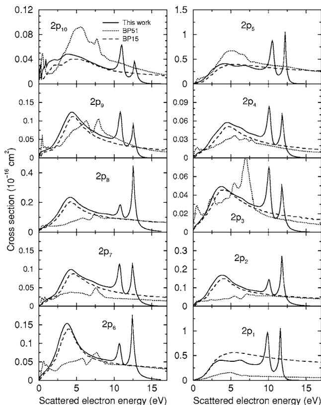
FIG. 4. The excitation cross sections from the ground level to the levels of  $4p^5 5p$  configuration as a function of scattered electron energy (solid lines, this work). The dotted lines represent 51-state BP  $R$ -matrix calculation obtained by Dasgupta *et al.* [18]; dashed lines, 15-state BPRM results [18].
