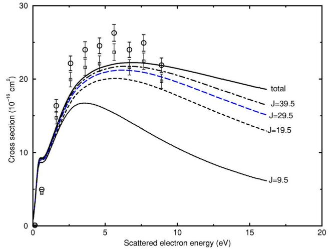
FIG. 1. (Color online) The convergence trend of excitation cross sections of transition  $1s_5 \rightarrow 2p_6$  with the number of partial waves. The experimental data of Jung *et al.* [11] are denoted by circles with error bars being given, while the squares represent the experimental data reduced by 10% to correct the cascade contribution of higher levels.
