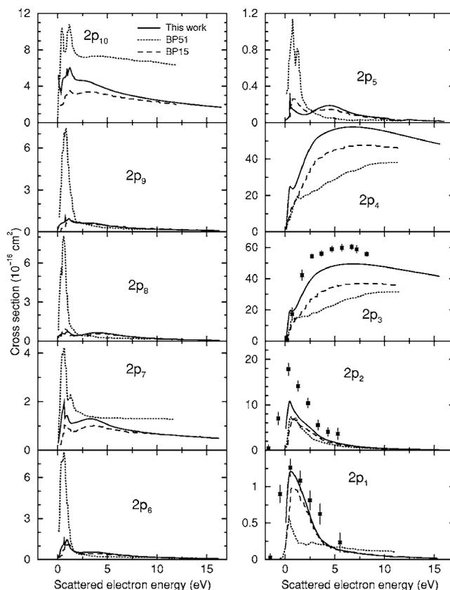
FIG. 7. The excitation cross sections from the metastable level  $1s_3$  to the levels of  $4p^55p$  configuration as a function of scattered electron energy (solid lines, this work). The dotted lines represent 51-state BP *R*-matrix calculation obtained by Dasgupta *et al.* [19]; dashed lines, 15-state BPRM results [19]. The circles are experimental results obtained by Jung *et al.* [11].
