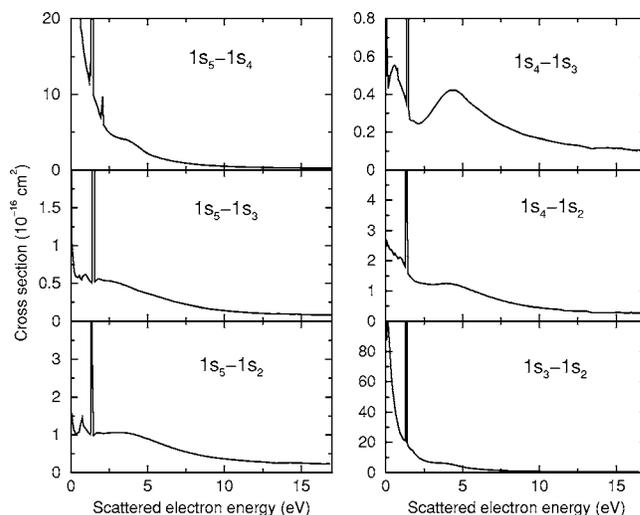
FIG. 9. The excitation cross sections for transitions between the levels of  $4p^55s$  configuration:  $1s_5-1s_4$ ,  $1s_5-1s_3$ ,  $1s_5-1s_2$ ,  $1s_4-1s_3$ ,  $1s_4-1s_2$ , and  $1s_3-1s_2$ .
