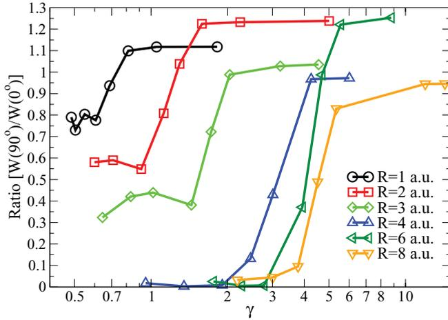
FIG. 3. (Color online) Ratios of ionization rate  $[W(90^\circ)/W(0^\circ)]$  versus the Keldysh parameter for the  $1\sigma_g$  state of  $H_2^+$ . The internuclear separations are 1 a.u. ( $\circ$ - $\circ$ ), 2 a.u. ( $\square$ - $\square$ ), 3 a.u. ( $\diamond$ - $\diamond$ ), 4 a.u. ( $\triangle$ - $\triangle$ ), 6 a.u. ( $\blacktriangleleft$ - $\blacktriangleleft$ ), and 8 a.u. ( $\nabla$ - $\nabla$ ). The laser carrier wavelength  $\lambda = 800$  nm.
