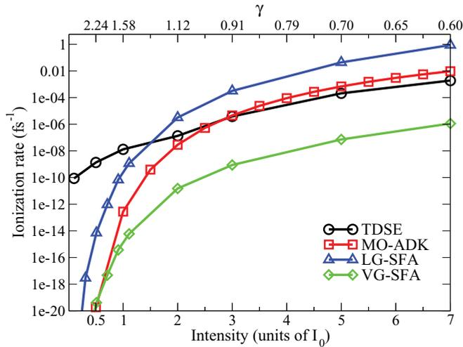
FIG. 6. (Color online) Ionization rate versus laser intensity when  $\theta = 0^\circ$  for the  $1\sigma_g$  state of  $H_2^+$  ( $R = 2$  a.u.). The rates are calculated from TDSE ( $\circ$ - $\circ$ ), MO-ADK ( $\square$ - $\square$ ), LG-SFA ( $\triangle$ - $\triangle$ ), and VG-SFA ( $\diamond$ - $\diamond$ ), respectively. The corresponding  $\gamma$  value is shown on the upper scale. The laser wavelength is 800 nm.
