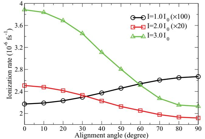
FIG. 2. (Color online) Normalized (to the maximum) ionization rates versus alignment angle  $\theta$  when the internuclear distance  $R = 2$  a.u. for the  $1\sigma_g$  state of  $H_2^+$ . The laser intensities are  $1.0I_0$  ( $\circ$ - $\circ$ ,  $\times 100$ ),  $2.0I_0$  ( $\square$ - $\square$ ,  $\times 20$ ), and  $3.0I_0$  ( $\triangle$ - $\triangle$ ), respectively. The laser carrier wavelength is 800 nm.
