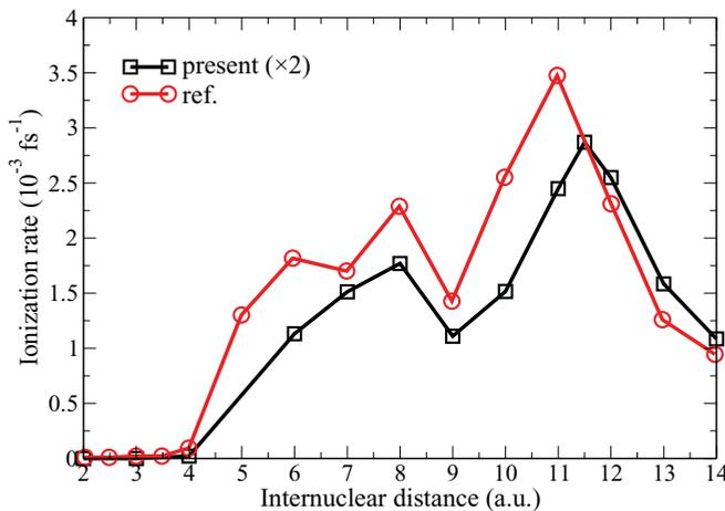
FIG. 4. (Color online) Ionization rate versus internuclear distance for  $1\sigma_g$  state of  $H_2^+$ , when laser field polarization direction lies parallel to molecular axis ( $\theta = 0^\circ$ ). The laser-field peak intensity and carrier wavelength are  $0.5I_0$  and 800 nm, respectively, for the present calculation ( $\square$ - $\square$ ,  $\times 2$ ), while comparable parameters of  $0.6I_0$  and 790 nm are used for the reference data [38] ( $\circ$ - $\circ$ ).
