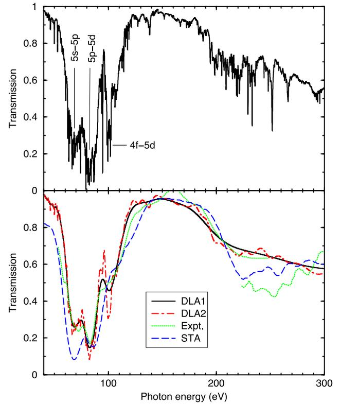
FIG. 2. (Color online) The same as in Fig. 1, while extensive core-valence electron correlations have been included in the calculation of bound-bound transitions: (a) DLA results and (b) with instrumental broadening included. In this figure, the physical effects such as core-valence correlations and autoionization widths have been considered, while in Fig. 1, these effects have not been included.
