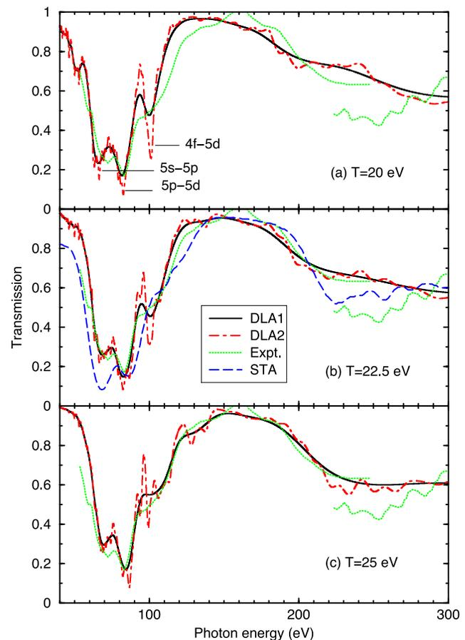
FIG. 3. (Color online) Transmission of Au plasmas at a density of  $0.007 \text{ g/cm}^3$  and temperatures of (a) 20, (b) 22.5, and (c) 25 eV, respectively.
