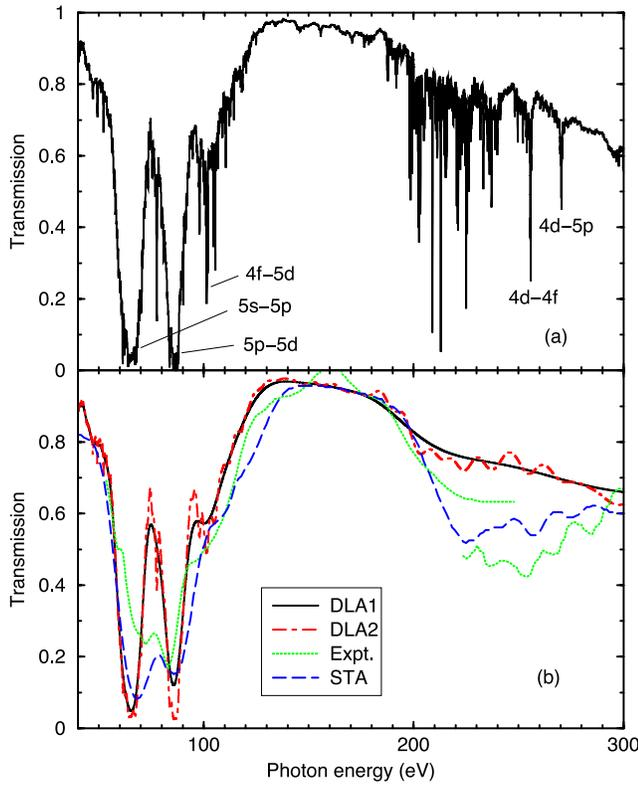
FIG. 1. (Color online) Transmission of a Au plasma at a temperature of 22.5 eV and a density of 0.007 g/cm<sup>3</sup>: (a) DLA results and (b) with instrumental broadening included. The experimental and STA data are taken from Ref. [8].
