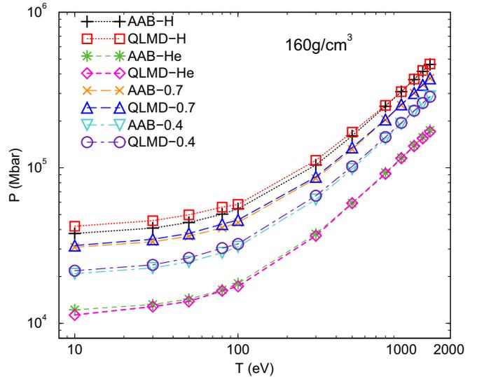
**Figure 4.** Pressure vs. temperature for a density of  $160 \text{ g cm}^{-3}$  with different chemical compositions compared with the results of AAB.
