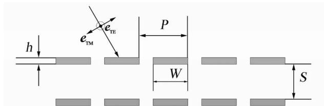
Fig. 1. DGP: rectangles filled with gray color, metal wires;  $P$ , wire period;  $S$ , spacing between two layers of gratings;  $h$ , wire depth; and  $w$ , metal wire width.
