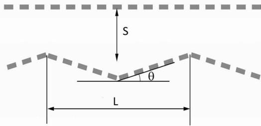
Fig. 7. Geometric depiction for corrugated DGP:  $\theta$ , inclination angle;  $L$ , corrugation period;  $S$ , spacing of original parallel gratings.
