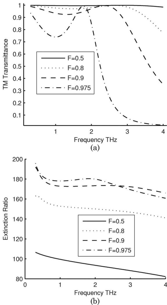
Fig. 4. (a) TM transmittance and (b) extinction ratio for DGP with various fill factors. The spacing is  $25\ \mu\text{m}$ , the period is  $5\ \mu\text{m}$ , and the wire depth is  $1\ \mu\text{m}$ .
