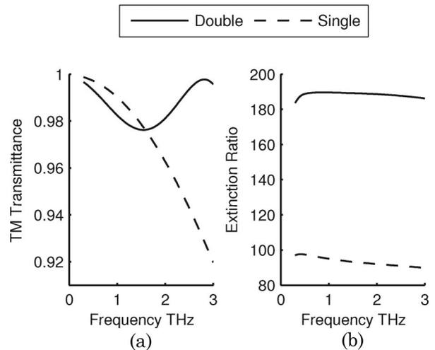
Fig. 5. (a) TM transmittance and (b) extinction ratio for DGP (solid curve) and SGP (dotted curve) with optimized geometric parameters (period of  $3\ \mu\text{m}$ , fill factor of 0.8, wire depth of  $1\ \mu\text{m}$ , and spacing of  $24\ \mu\text{m}$ ).
