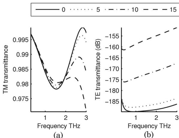
Fig. 8. (a) TM and (b) TE transmittance spectra for corrugated DGP with inclination angles of 0°, 5°, 10°, and 15°. The grating period is  $3\mu\text{m}$ , the fill factor is 0.8, parallel spacing is  $24\mu\text{m}$ , and wire depth is  $1\mu\text{m}$ .
