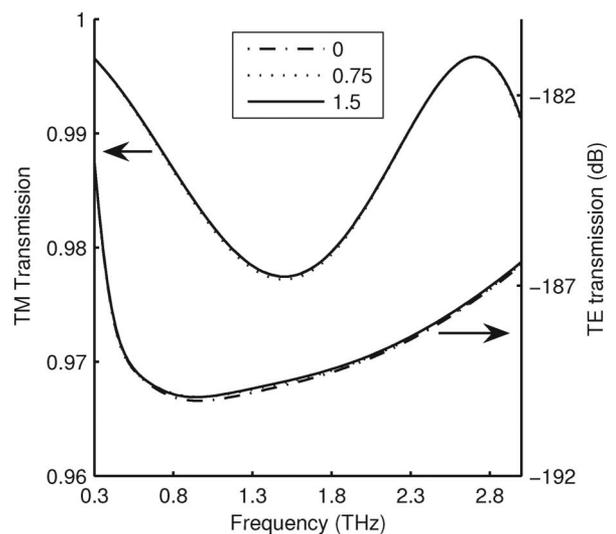
Fig. 6. TM and TE transmittance through optimized DGP with various lateral shifts. Dashed-dotted curve is of zero lateral shift, dotted curve is of  $0.75\ \mu\text{m}$  lateral shift (a quarter of the period), and solid curve is of  $1.5\ \mu\text{m}$  lateral shift (half of the period).
