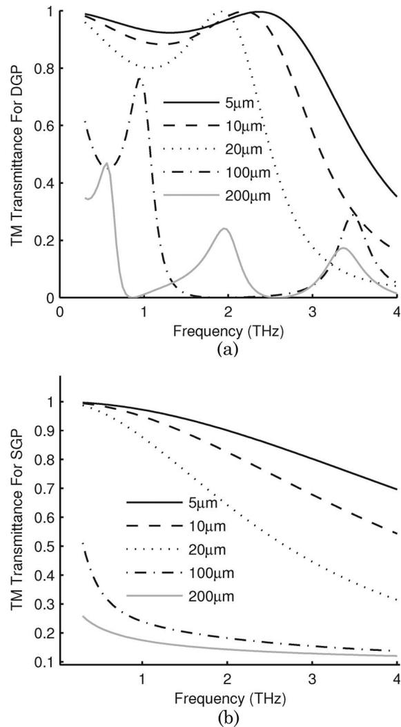
Fig. 3. TM transmittance spectra for  $5\ \mu\text{m}$ ,  $10\ \mu\text{m}$ ,  $20\ \mu\text{m}$ ,  $100\ \mu\text{m}$ , and  $200\ \mu\text{m}$  periods. (a) Spectra of DGP. (b) Spectra of corresponding SGP.
