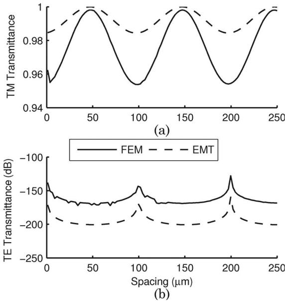
Fig. 2. (a) TM and (b) TE transmittance for DGP as a function of spacing. The wavelength is  $200\ \mu\text{m}$ , the fill factor is 0.8, and the wire depth is  $1\ \mu\text{m}$ . Solid curve, FEM result; dotted curve, EMT result.
